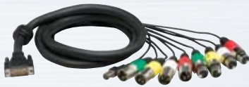
CBL-AES1604 Digital Input/Output Cable for AES16, AES16e DB26 to four female and four male XLR (8 mono AES output channels), and BNC (word clock I/O), 6 feet.
