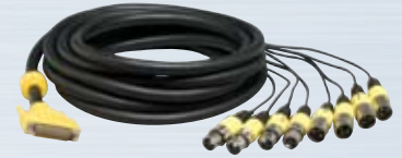
CBL-DIGY85 Digital Input/Output Cable Eight channels AES/EBU I/O. DB25 with four female and four male XLR connectors; 5 meters (16.4 feet); Yamaha pinout.
